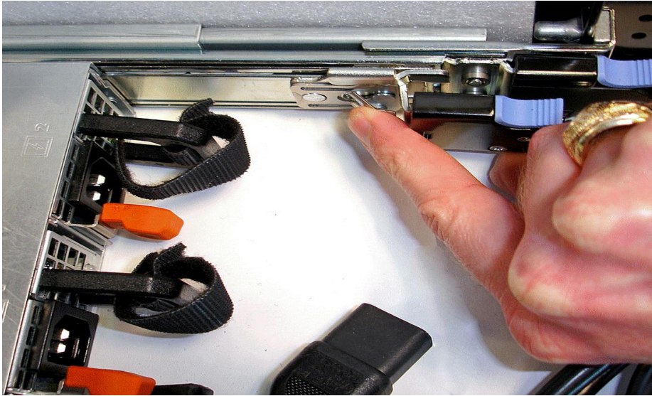
Figure 11: Replacing the Outer Power Supply
